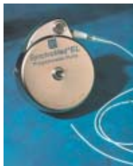
An example of a programmable drug delivery pump. The illustration shows the body of the pump with the spinal catheter connected to it.
