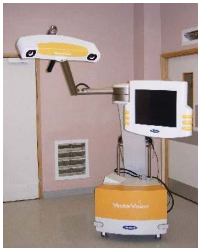
Figure 3: Neuronavigation equipment. The optical digitiser comprises LED emitters and infrared cameras. The touch screen monitor provides the surgeon with readily accessible software access.
