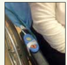
Image 5: Standard call bell attached to armrest operated by increased precision antigravity shoulder and elbow movement
