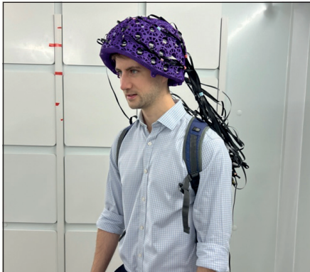
Figure 5: an example of a wearable OPM-MEG being used to investigate cortical activity at the Sir Peter Mansfield Imaging Centre, University of Nottingham
