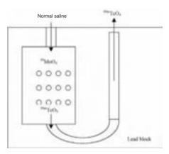
Figure 2a: Technetium-99m is produced from a generator which contains <sup>99</sup>MolybdenumO<sub>4</sub> adsorbed onto beads in column. The generator produces sufficient activity for about one week's supply of Tc-99m. The Tc-99m is eluted from the column by the addition of a solution of normal saline. The more soluble <sup>99m</sup>TCO<sub>4</sub> is preferentially released from the beads. The generator can be eluted once every six hours.
