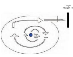
Figure 2b: Fluoride-18 and a neutron are produced by a cyclotron by the collision of Oxygen-18 with a proton.
